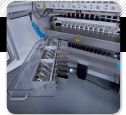
3. Independent rejection system.
