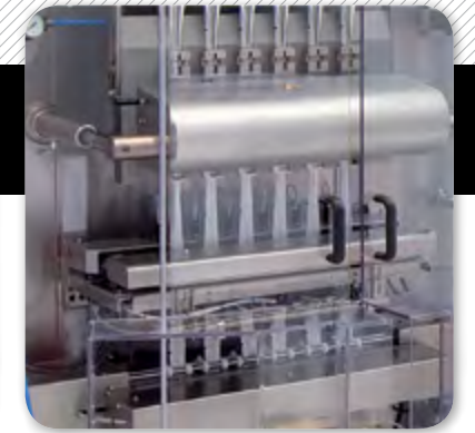
3. Independent sealing jaws.
